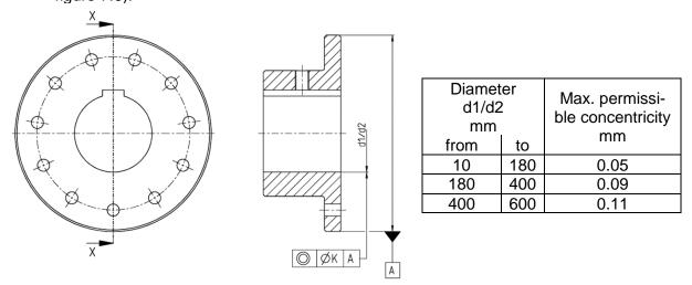
Figure 7.6: Form and positional tolerance of the bore and position of the keyway nut
