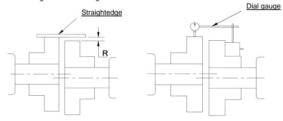
Figure 7.2: Measurement with a straightedge
