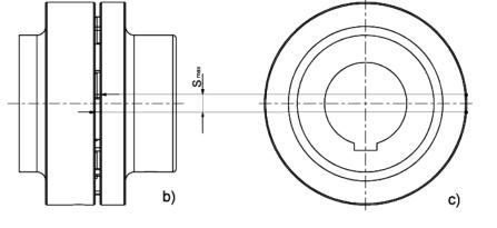
Figure 10.1: Check the wear limit
