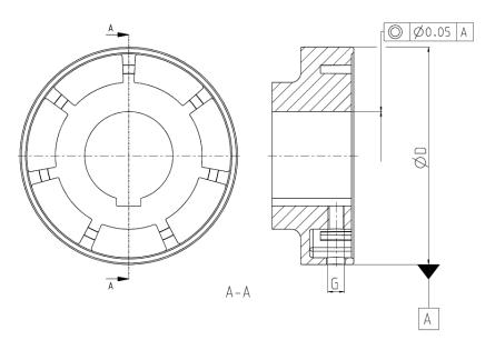
Figure 7.3: Specifications for the form and positional tolerance of the bore and position of the keyway nut
