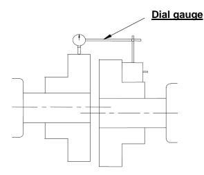
Figure 7.3: Measurement with a dial gauge
