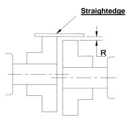
Figure 7.2: Measurement with a straightedge
