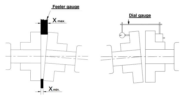
Figure 7.4: Measurement with a feeler gauge
